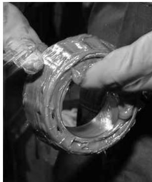
Fig. 51. Grease can easily be packed by hand.
